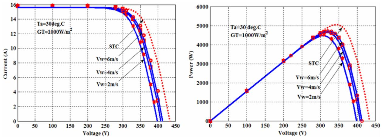
Figure 7. I-V curves (left) and P-V curves (right) for PV array versus experiment data (scattered points) at different wind speeds
