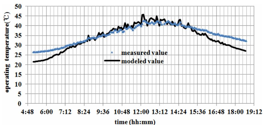
Figure 4. Comparison of measured with the modeled operating temperature values
