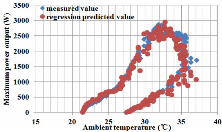
Figure 13. Regression predicted versus measured maximum power outputs at different ambient temperatures
