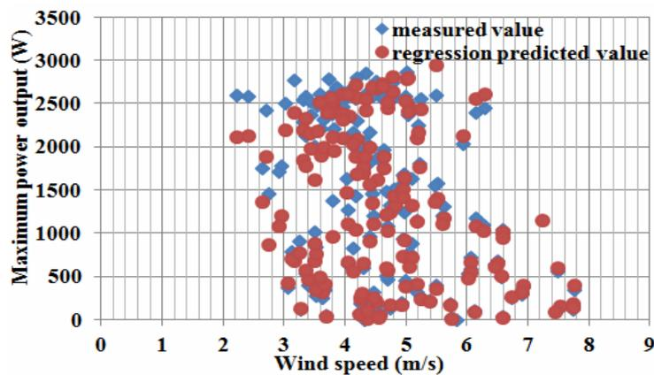
Figure 14. Regression predicted versus measured maximum power outputs at different wind speeds
