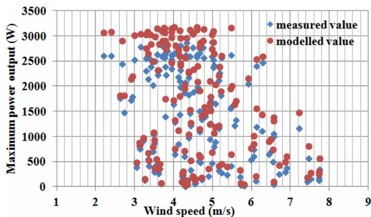
Figure 11. Modeled versus measured maximum power outputs at different wind speeds
