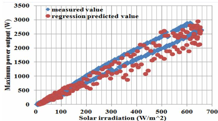
Figure 15. Regression predicted versus measured maximum power outputs at different irradiance
