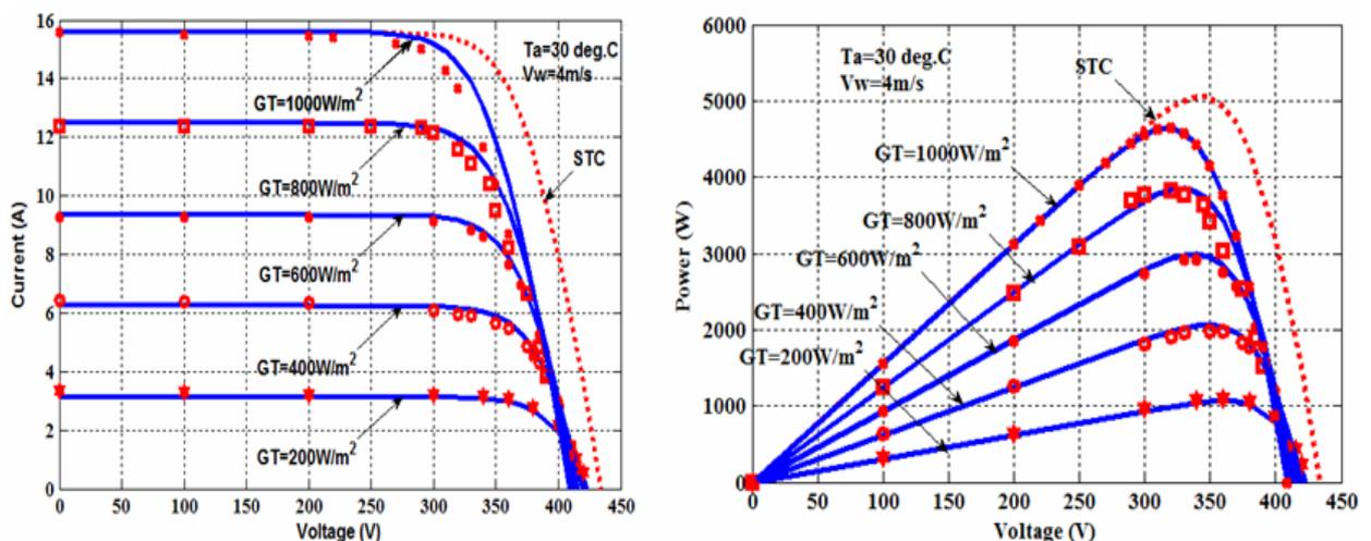
Figure 6.  $I-V$  curves (left) and  $P-V$  curves (right) for PV array versus experiment data (scattered points) at different irradiance
