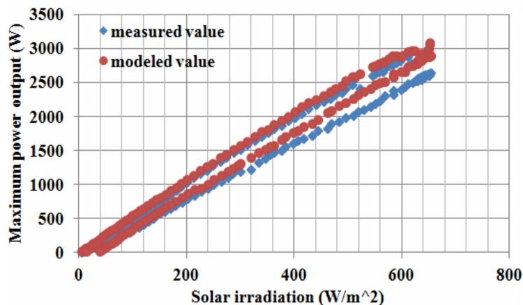
Figure 10. Modeled versus measured maximum power outputs at different irradiance
