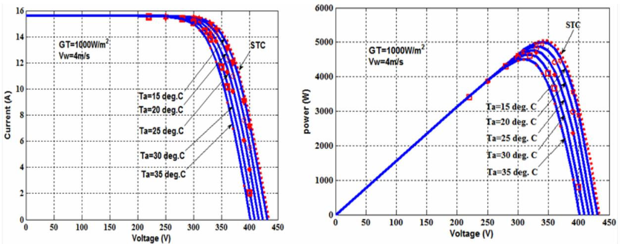
Figure 5.  $I-V$  curves (left) and  $P-V$  cures (right) for PV array versus experiment data (scattered points) at different ambient temperatures
