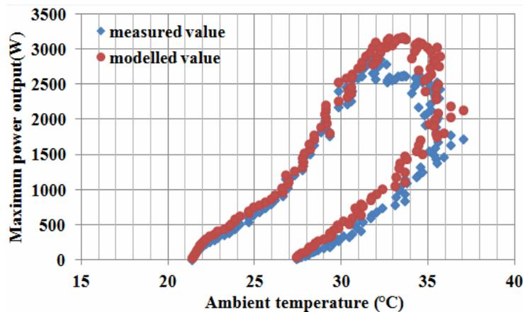
Figure 9. Modeled versus measured maximum power outputs at different ambient temperatures
