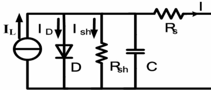
Figure 1. Equivalent circuit for photovoltaic cell
