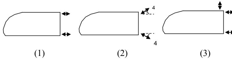
Figure 14. Three oscillatory jet configurations employed in the drag reduction study [9]
