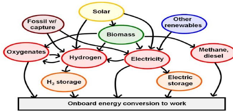
Figure 30. Fuel chain possibilities for carbon free energy for transportation [15]
