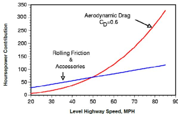
Figure 12. Variation in aerodynamic drag and rolling resistance with speed [6]
