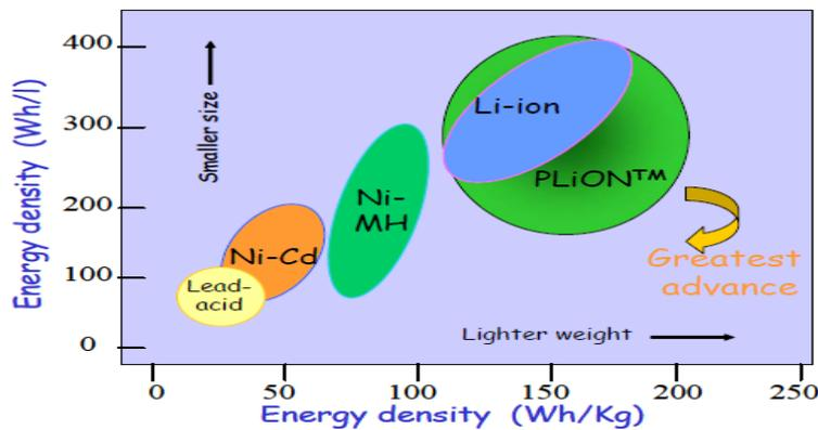
Figure 32. Current state of the battery performance metric [16]
