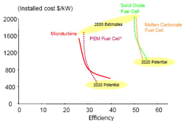
Figure 34. Various types of fuel cells, their cost and efficiency
