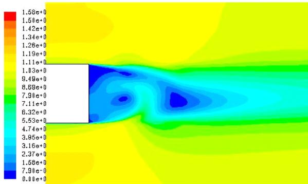
Figure 17. Velocity contours without AFC for  $Re = 3.08 \times 10^5$  [9]
