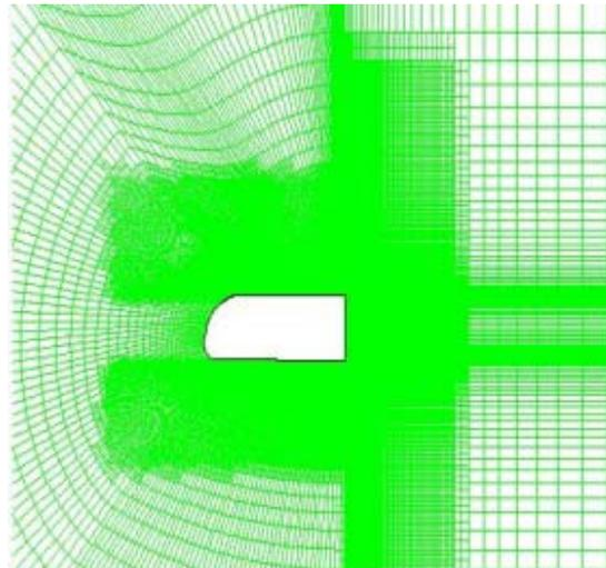
Figure 15. Adaptive mesh around the 2D truck [9]
