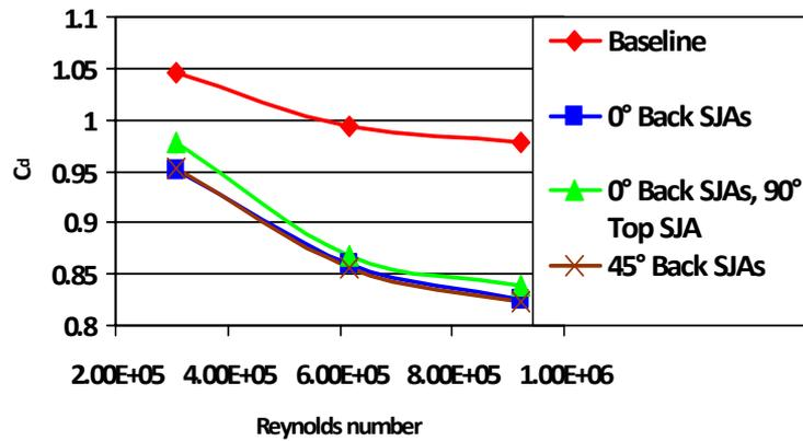
Figure 19. Variation of drag coefficient with Reynolds number without and with AFC [9]
