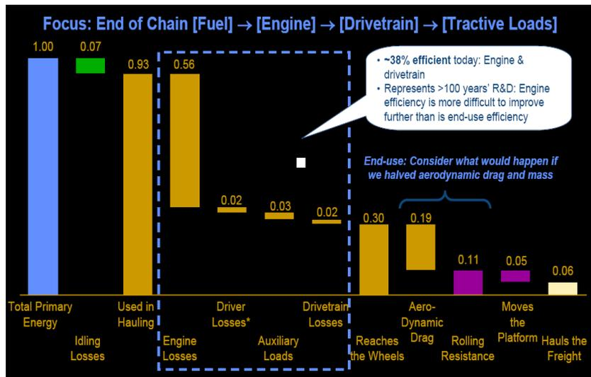
Figure 9. Expenditure of fuel energy in a typical class 8 truck of weight ~ 35,000 lbs. [5]
