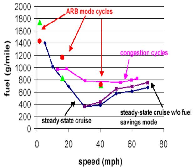
Figure 24. Effect of congestion on fuel efficiency [11]
