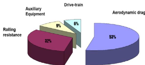
Figure 10. Main sources of energy losses from available mechanical power from the engine [2]
