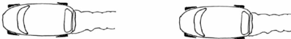
Figure 20. The second vehicle experiences the wake of the first vehicle (with lower dynamic pressure) resulting in lower total drag for the two vehicles [6]
