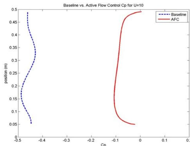
Figure 16. Static pressure at the rear face of the truck; Blue – without AFC, Red – with AFC for case 1 of Figure14 [9]
