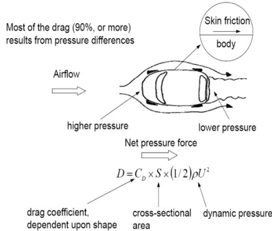
Figure 11. Shape and speed contributing to the aerodynamic drag of a vehicle [6]
