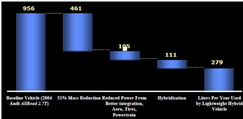
Figure 25. Effect of mass reduction and other technologies on fuel consumption of a typical SUV for a typical driving pattern in U.S. [5]
