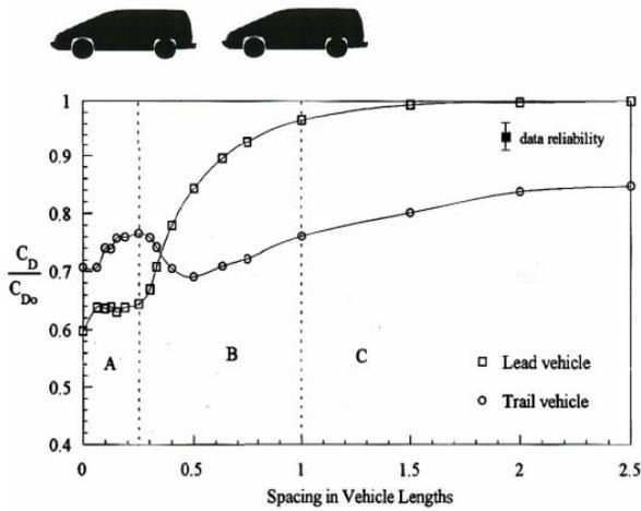
Figure 21. Variation in drag coefficient of two identical vehicles as a function of spacing between them [6]
