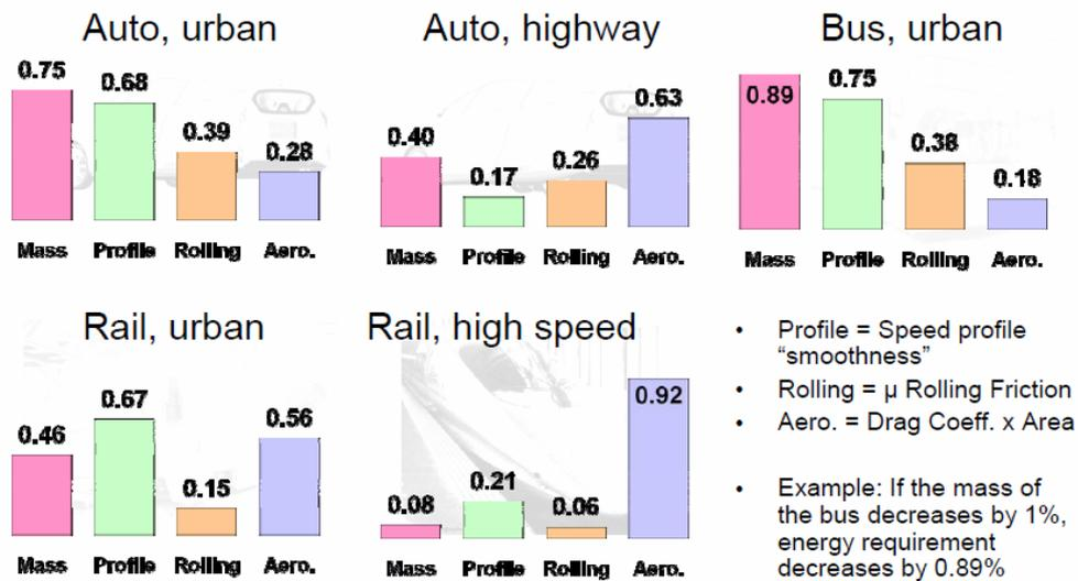
Figure 26. Propulsive energy requirement sensitivity of automobiles, buses, and rails with respect to mass, speed profile smoothness, rolling resistance and drag [13]
