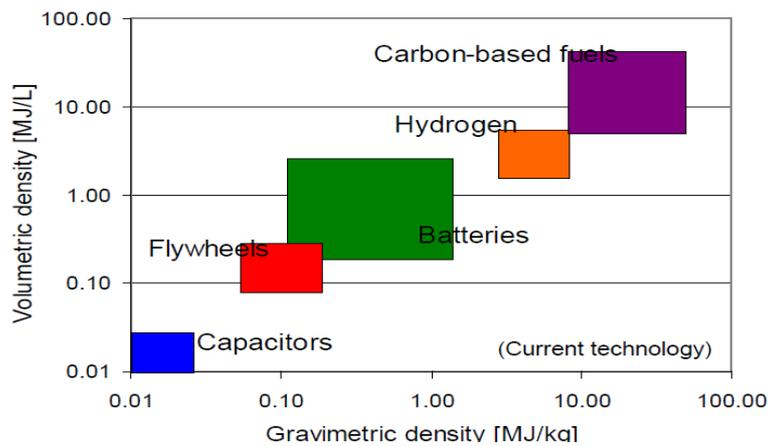
Figure 31. Energy storage density of various energy storage devices [13]
