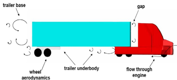
Figure 13. Critical flow separation regions surrounding a heavy duty truck which contribute to drag [2]
