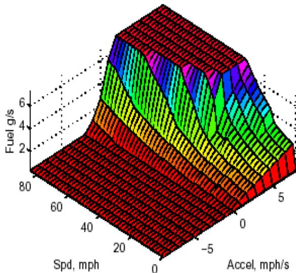
Figure 23. Effect of speed variation on fuel efficiency [11]
