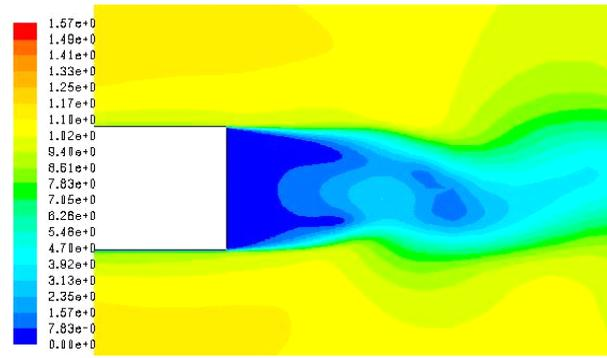
Figure 18. Velocity contours with AFC for  $Re = 3.08 \times 10^5$  for case 1 of Figure 14 [9]
