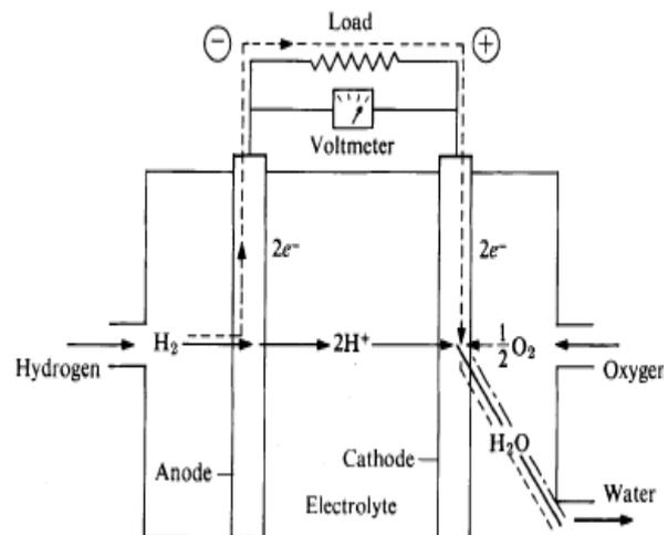
(b) Operation schematic of a fuel cell
