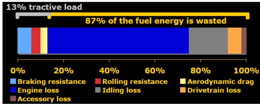
Figure 8. Expenditure of fuel energy in a typical automobile [5]
