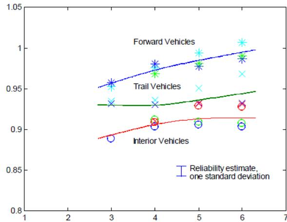
Figure 22. Variation in drag coefficient of three identical vehicles as a function of spacing between them [6]
