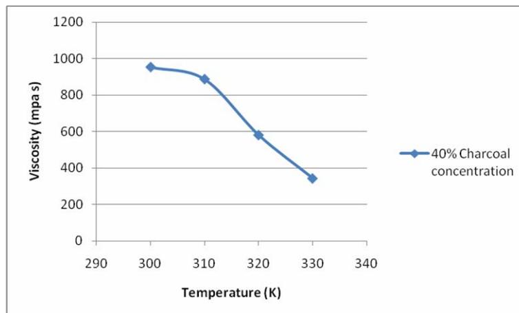
Figure 4. Viscosity temperature relationship for charcoal-water slurry (40% w/w)
