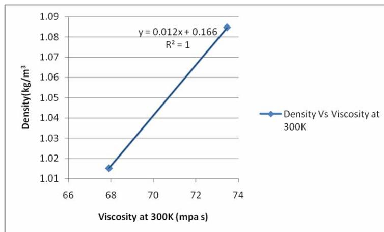
Figure 5. Correlation between density and viscosity
