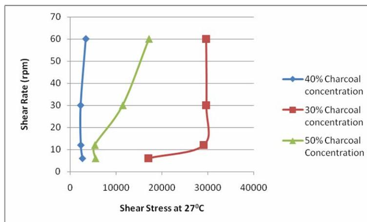
Figure 2. Shear stress vs shear rate
