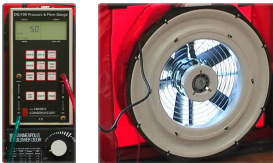
Figure 2. Minneapolis model 3 blower unit and a DG-700 digital gauge
