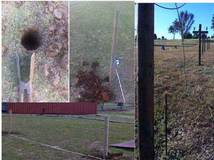
Figure 4. UWS field test area and the single electrode installation
