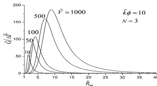
Figure 8. Effect of  $\tilde{V}$  on  $\tilde{G}/\Delta\tilde{T}$  versus  $\tilde{R}_{out}$  with fixed  $\tilde{k}\phi$  and  $N$
