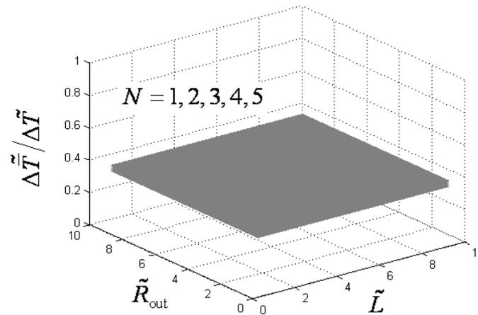
Figure 13.  $\tilde{\Delta T}/\Delta T$  corresponding to different  $N$  versus  $\tilde{L}$  and  $\tilde{R}_{out}$
