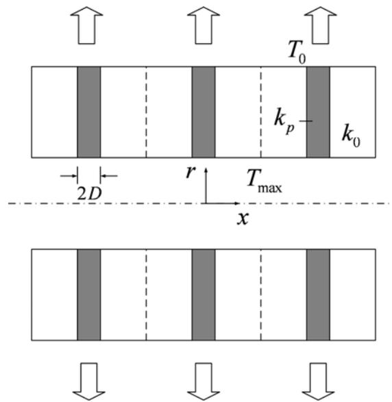
Figure 2. Solenoid cooled by transversal discs with high thermal conductivity [65]
