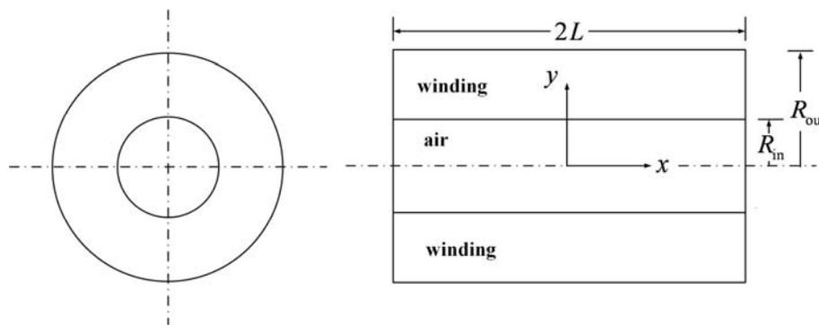
Figure 1. The main features of solenoid geometry [65]
