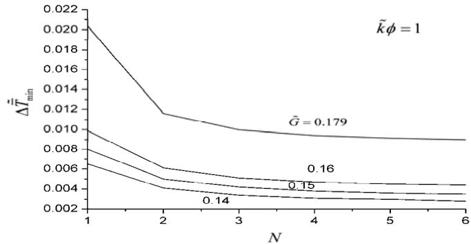
Figure 3. Effect of  $\tilde{G}$  on  $\Delta\tilde{T}_{min}$  versus  $N$  with fixed  $\tilde{k}\phi$  [66]
