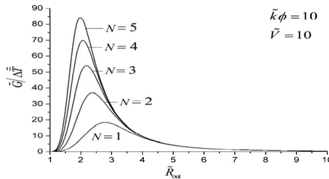
Figure 4. Effect of  $N$  on  $\tilde{G}/\Delta\tilde{T}$  versus  $\tilde{R}_{out}$  with fixed  $\tilde{k}\phi$  and  $\tilde{V}$
