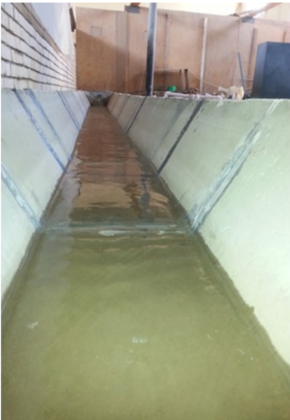
Figure 6. Trapezoidal canal with 5 CFRP sheets
