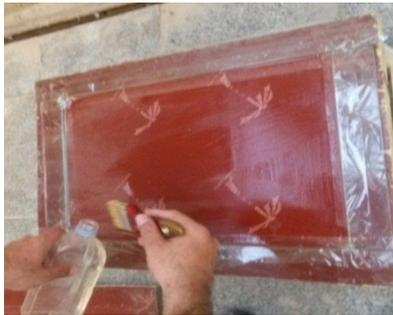
4- Painting the insulated layer on the wood block and glass frame
