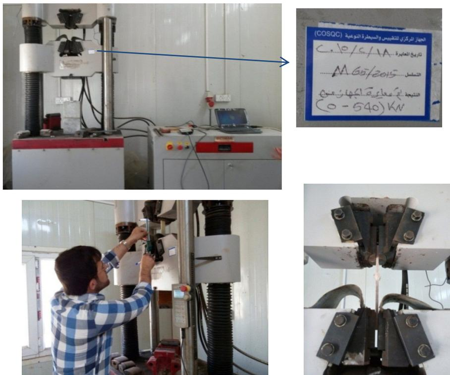
Figure 6. Tensile test machine and processes of test
