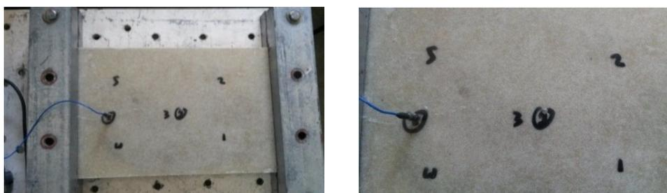
Figure 16. The central and lateral positions of e- accelerometer part on the vibration tested plat
