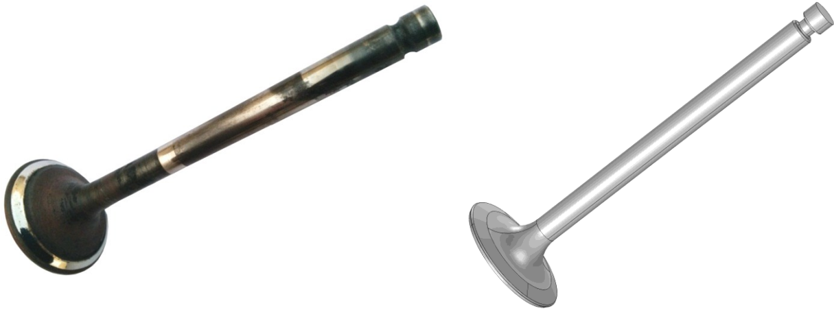
Figure 2. Real and three dimensional computational domains of the exhaust valve.
