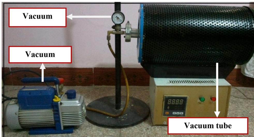
Figure 1. Electrical tube furnace.
