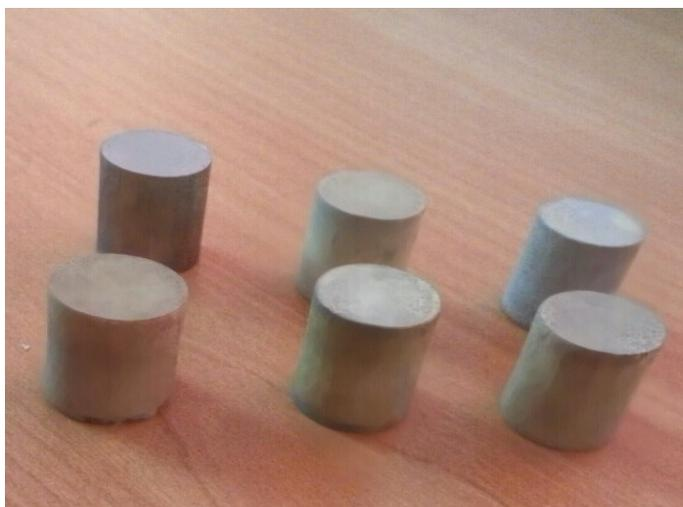
Figure 2. Samples after sintering.
