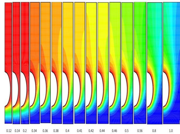
Figure 10. Temperature contour with various spacing between the tubes for ( $Ra=10^3, Pr = 0.7$  and axis ratio  $\epsilon = 0.25$ ).
