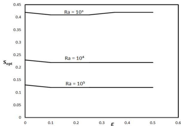
Figure 17. Optimum spacing with different axis ratios for Rayleigh Number.
