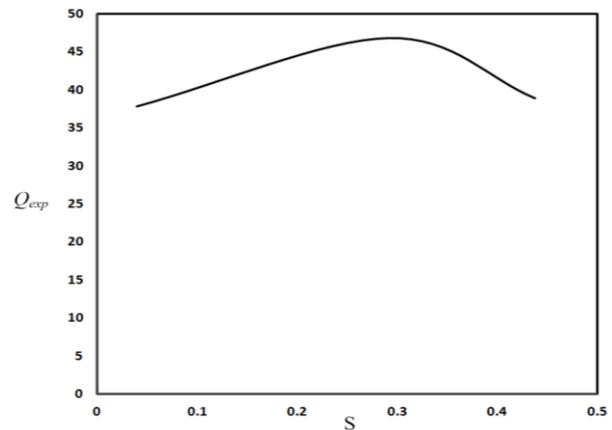
Figure 18. Experimental heat transfer density as a function of the spacing ( $S$ ) between the tubes for ( $Ra = 3.5 \times 10^4$ ) and ( $\epsilon = 0.25$ ).
