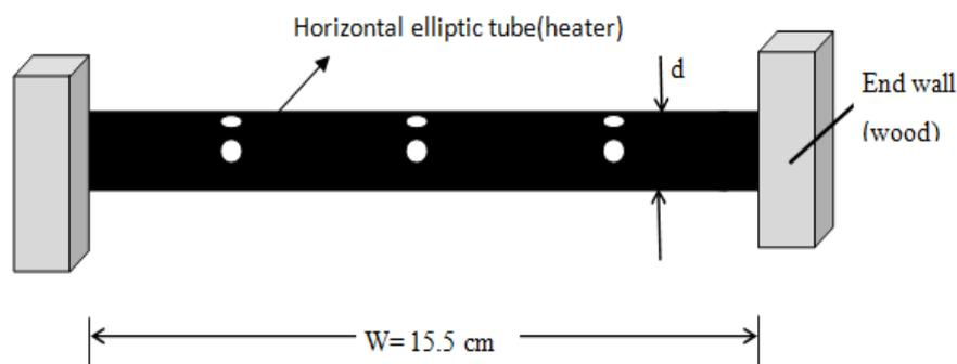
Figure 6. Position of the thermocouples on the elliptic tube
