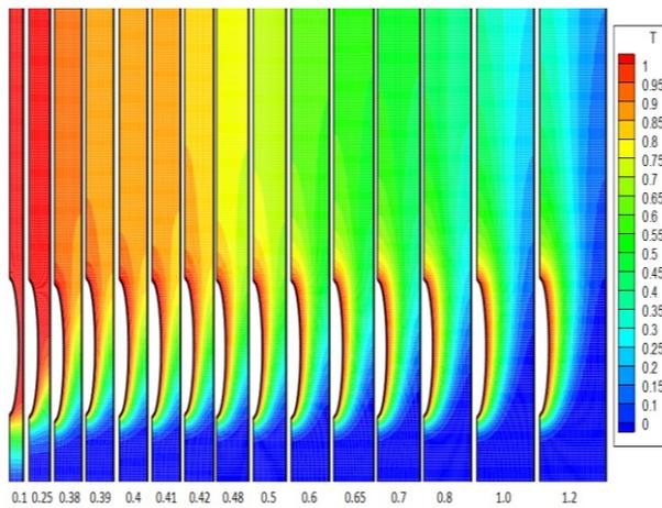
Figure 7. Temperature contour with various spacing between the tubes for ( $Ra=10^3, Pr = 0.7$  and axis ratio  $\epsilon = 0.1$ ).
