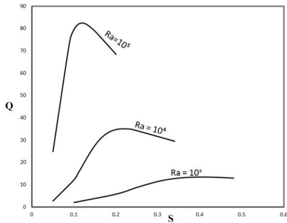
Figure 13. Heat transfer density with spacing at difference Rayleigh number for axis ratio  $\epsilon=0.1$ .
