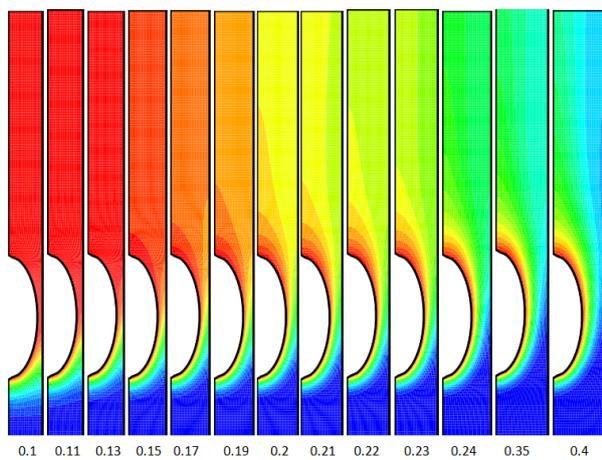
Figure 11. Temperature contour with various spacing between the tubes for ( $Ra=10^4, Pr = 0.7$  and axis ratio  $\epsilon = 0.25$ ).
