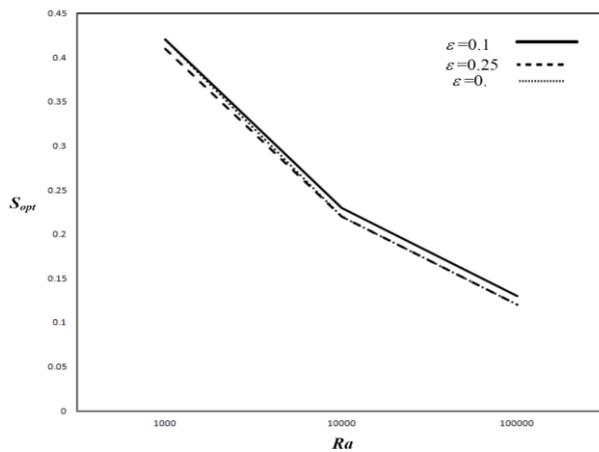
Figure 15. Optimum spacing with Rayleigh number of different axis Ratios.
