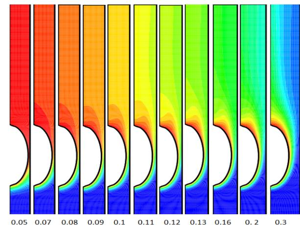
Figure 12. Temperature contour with various spacing between the tubes for ( $Ra=10^5, Pr = 0.7$  and axis ratio  $\epsilon = 0.25$ ).
