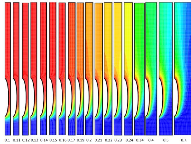
Figure 8. Temperature contour with various spacing between the tubes for ( $Ra=10^4, Pr = 0.7$  and axis ratio  $\epsilon = 0.1$ ).
