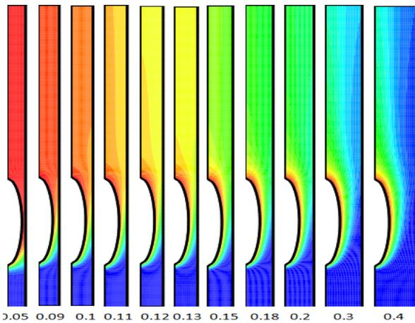
Figure 9. Temperature contour with various spacing between the tubes for ( $Ra=10^5, Pr = 0.7$  and axis ratio  $\epsilon = 0.1$ ).
