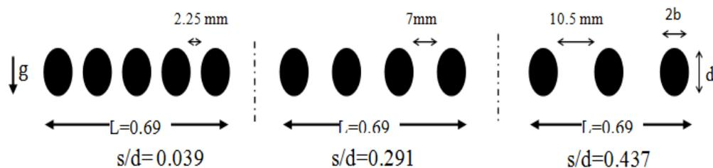
Figure 5. Details of main parts of the rows used in the experimental apparatus.
