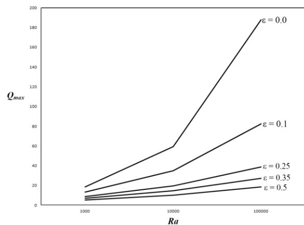
Figure 16. Maximum heat transfer density with Rayleigh number for different axis ratios.
