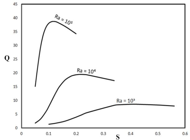
Figure 14. Heat transfer density with spacing at difference Rayleigh number for axis ratio  $\epsilon=0.25$ .
