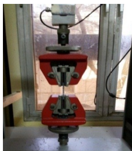
Figure 3. Material testing machine Testometric.
