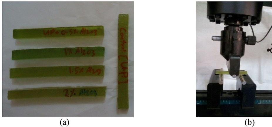
Figure 4. The bending test: (a) the samples are ready for bending test, (b) During the inspection: the edges of a specimen are carried on the test machine.
