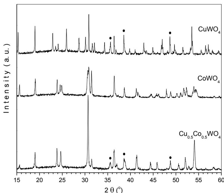
Figure 1. XRD patterns of  $\text{CoWO}_4$ ,  $\text{CuWO}_4$  and  $\text{Cu}_{0.5}\text{Co}_{0.5}\text{WO}_4$ . Peaks relating to copper oxide (●).
