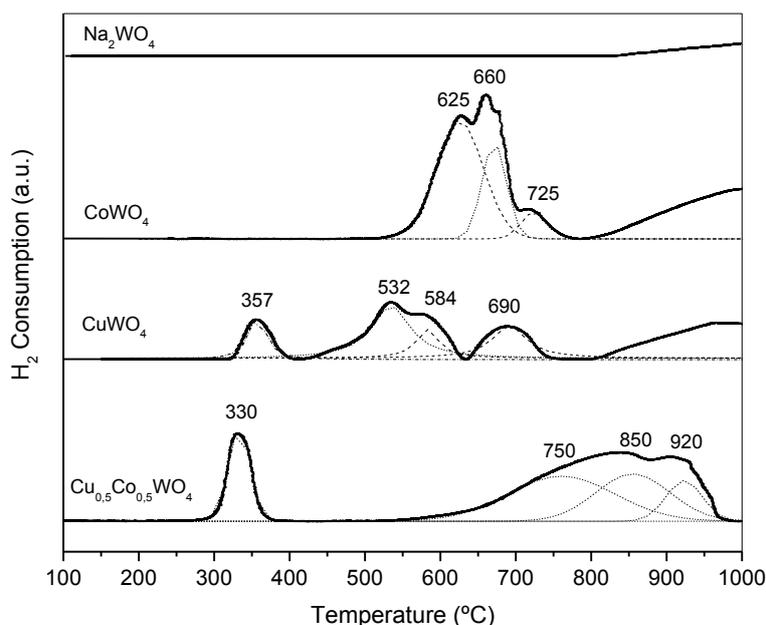
Figure 2. H<sub>2</sub>-TPR profiles of tungstate samples.
