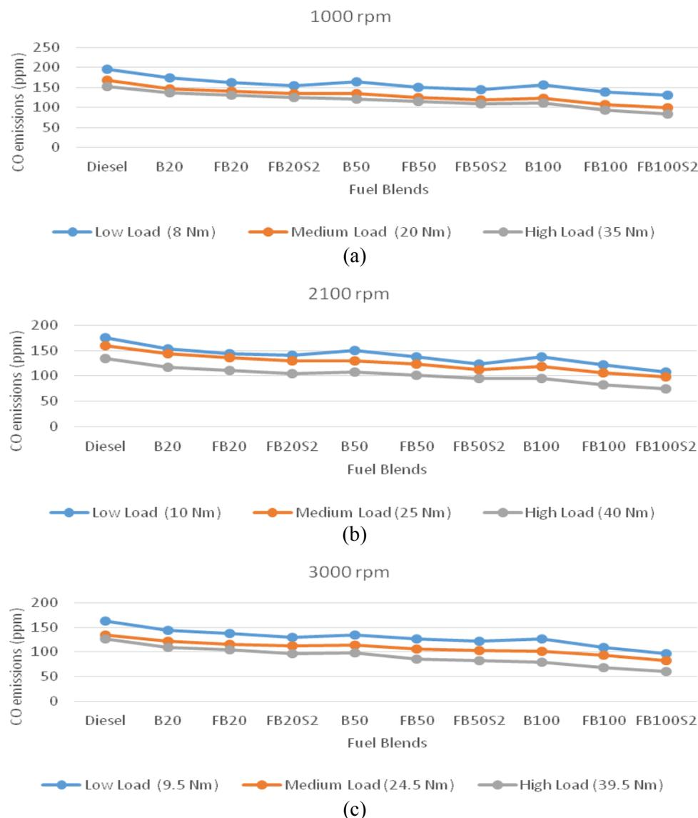
Figure 6. CO emissions at (a) 1000 rpm (b) 2100 rpm (c) 3000 rpm for different fuel blends under variable engine loads.
