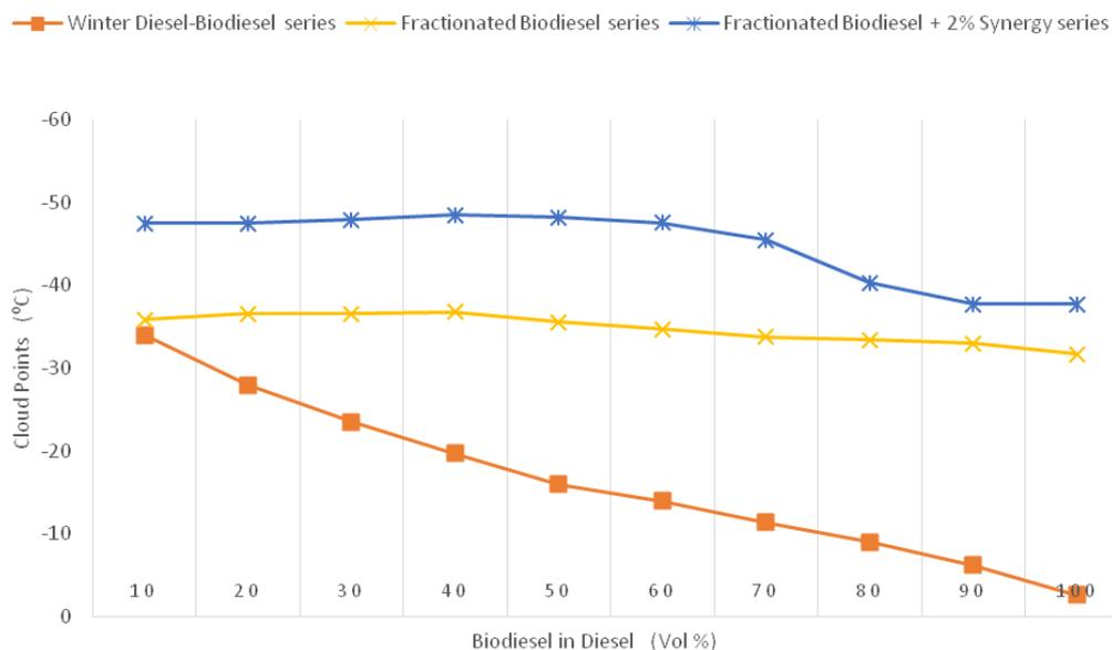
Figure 3. Variation of biodiesel content in diesel fuel and corresponding cloud points.
