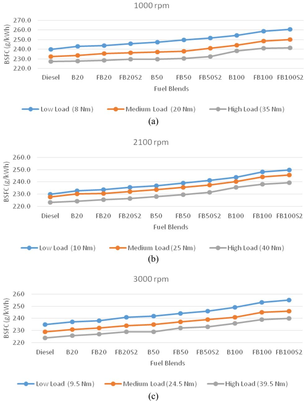
Figure 4. BSFC values at (a) 1000 rpm (b) 2100 rpm (c) 3000 rpm for different fuel blends under variable engine loads.
