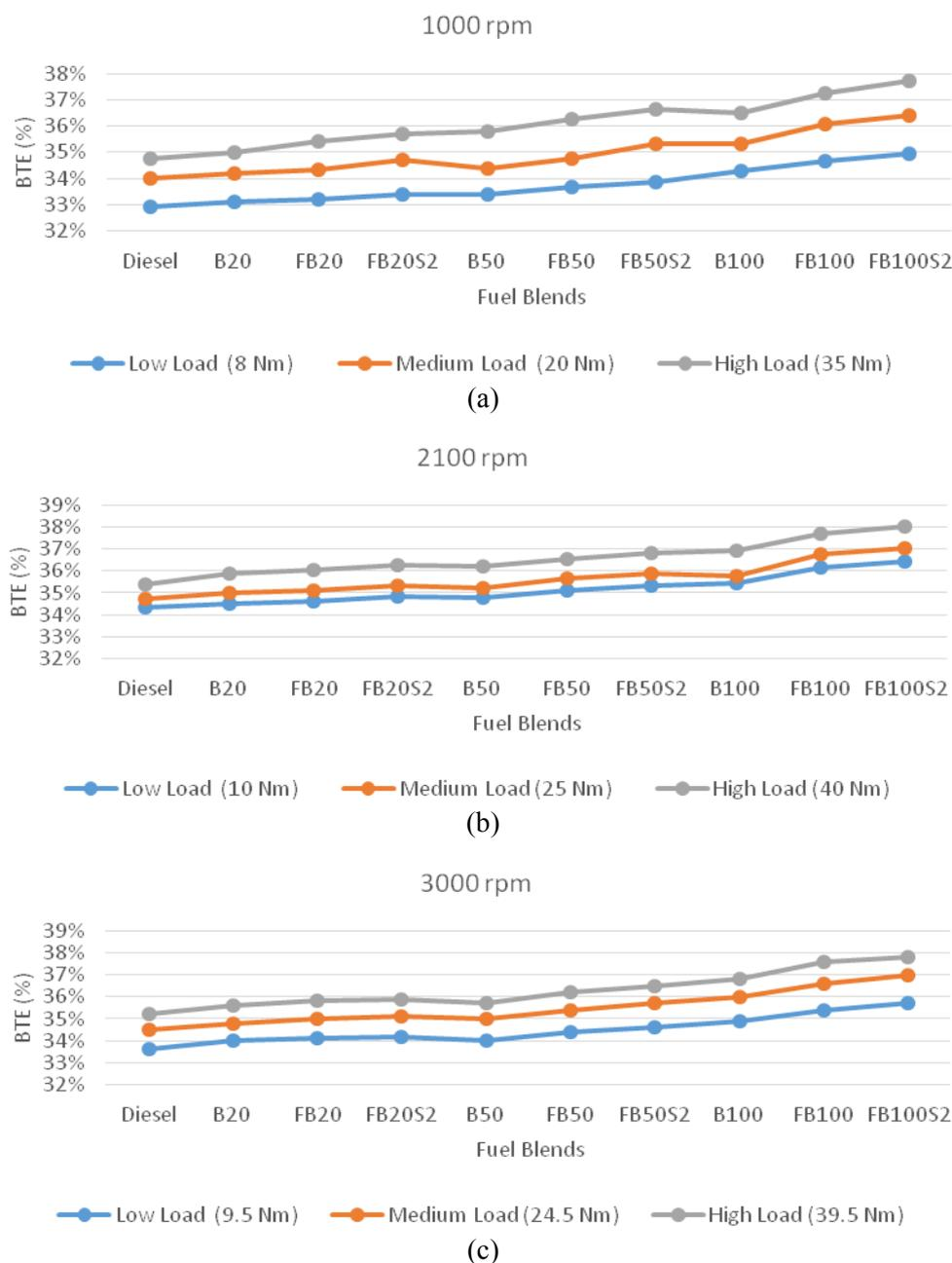
Figure 5. BTE values at (a) 1000 rpm (b) 2100 rpm (c) 3000 rpm for different fuel blends under variable engine loads.
