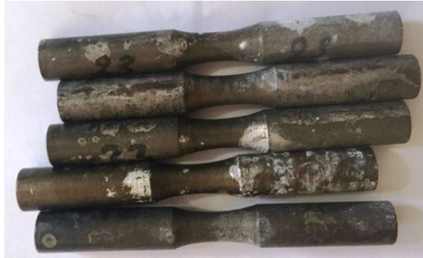
Figure 9. Example of fatigue specimens submerged in corrosive NaCl aqueous solution.
