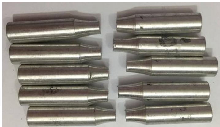
Figure 8. Fatigue specimens without UP after fatigue failure.
