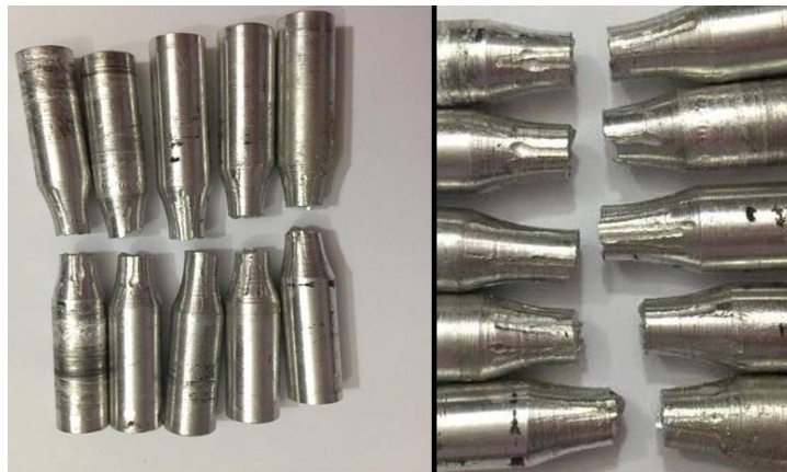
Figure 7. Fatigue specimens with UP after fatigue failure.
