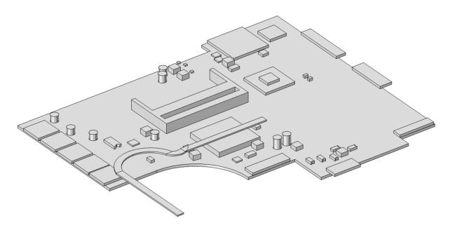
(b) three-dimensional computational domain with thermal management system (heat pipe).
