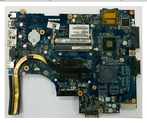
(a)  $hp^{\text{®}}$  motherboard with thermal management system (heat pipe).
