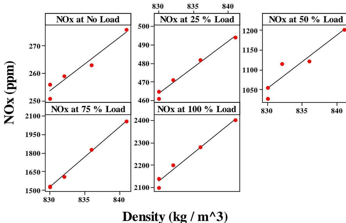
Figure 2.  $\text{NO}_x$  vs. density at different engine loads
