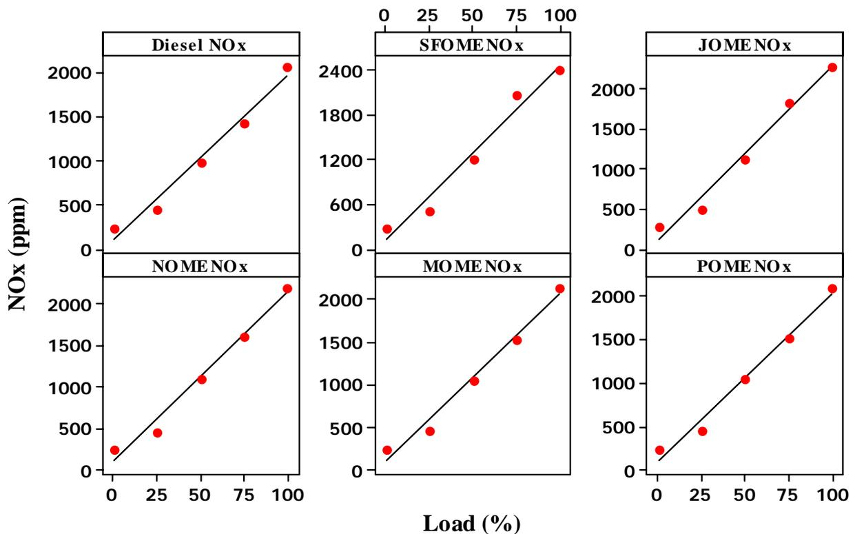
Figure 1. NO<sub>x</sub> Vs engine load for different biodiesel fuels
