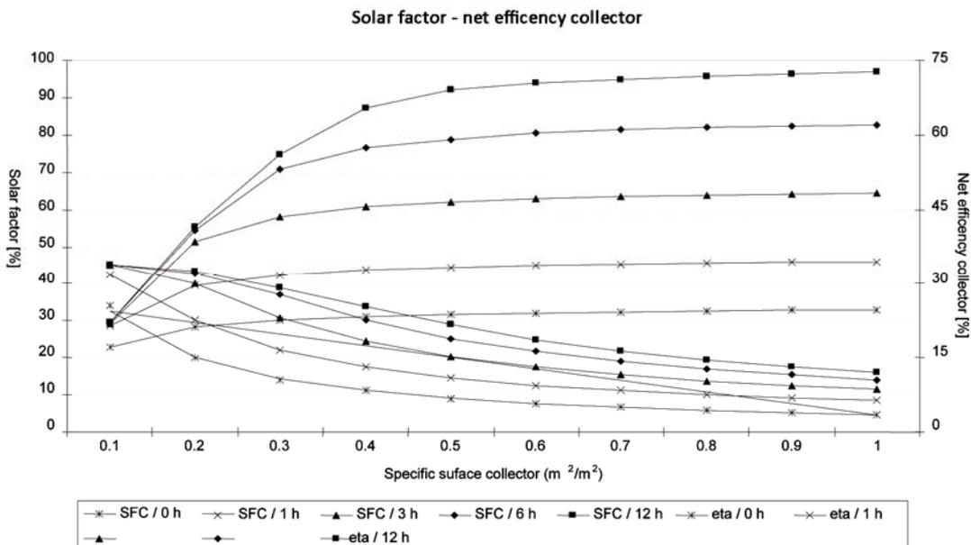
Figure 4. Solar factor and collectors net efficiency against the solar field surface
