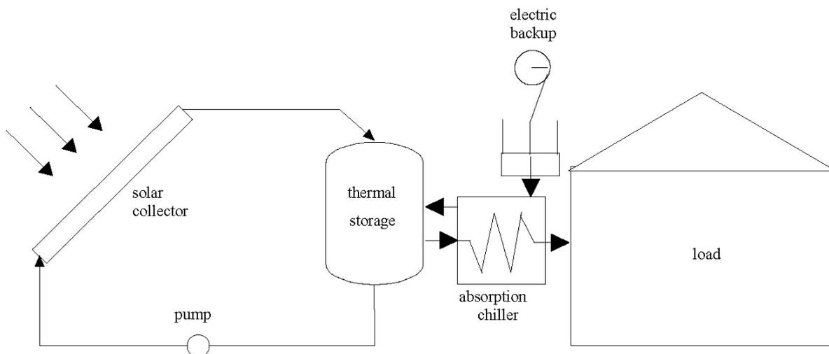
Figure 1. Absorption system scheme with electric backup
