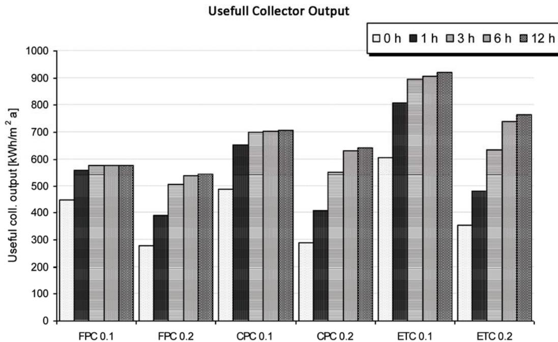
Figure 5. Useful annual energy produced by one  $m^2$  of collector against thermal storage typology system
