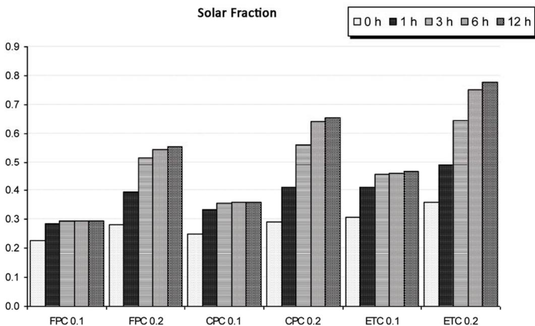
Figure 6. Solar factor against the collector type and the thermal storage capacity of the system
