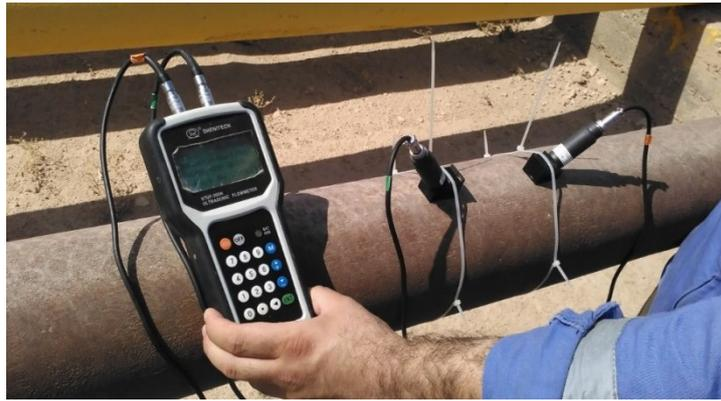
Figure 4. Ultrasonic Flow-meter.
