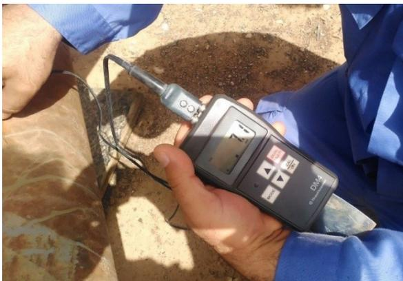
Figure 2. Ultrasonic thickness gauge.
