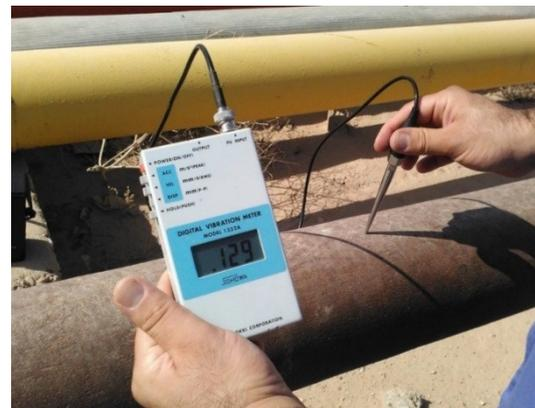
Figure 3. Digital vibration meter.
