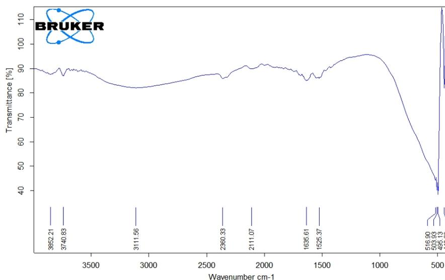
Figure 6. FT-IR for TiO<sub>2</sub> NPs.Table 3. The bonds of TiO<sub>2</sub>.
