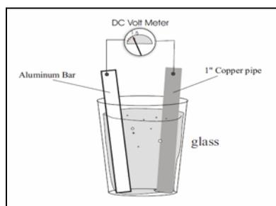
Figure 5. Arrangement of cell
