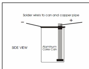
Figure 6. Sealing the cell
