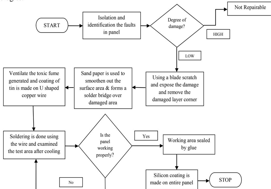
Figure 11. The flowchart of repairing damaged panel
