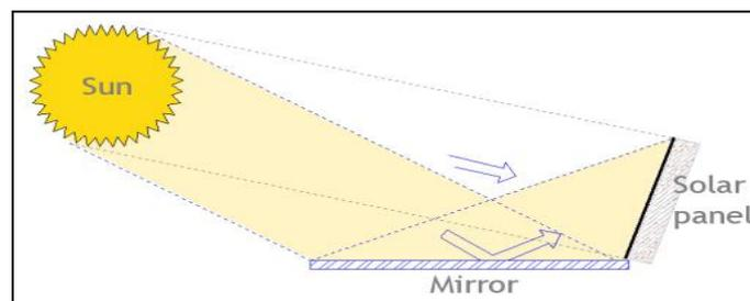
Figure 10. Use of reflecting media with solar panel
