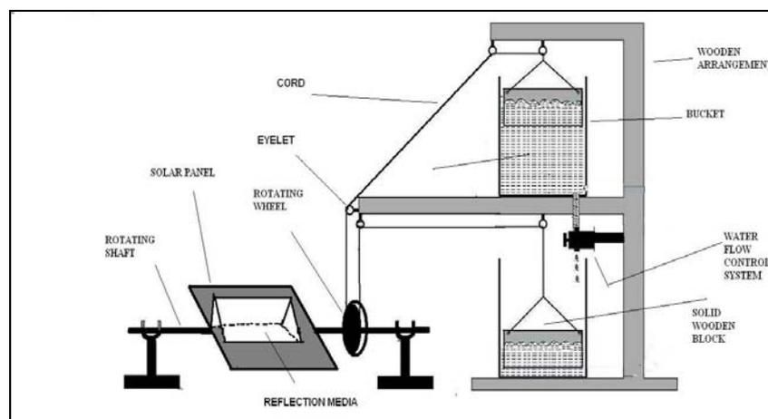
Figure 8. The working model of the alternative tracker system
