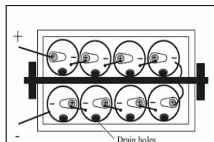
Figure 7. Arrangement of 8 such cells to form the battery
