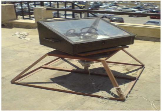
Figure 1. The tracking system of the solar cooker
