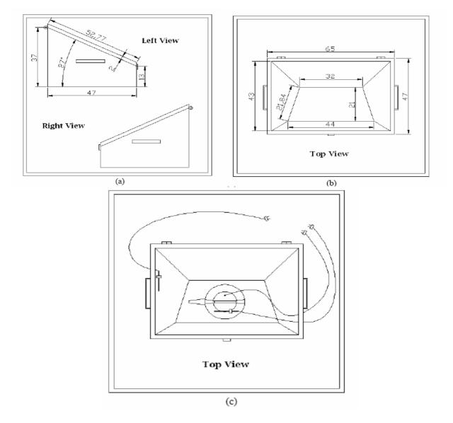
Figure 2. Three dimensional views of the designed solar cooker, (a) and (b) are cooker dimensions in cm, and (c) thermocouple connections in the cooker
