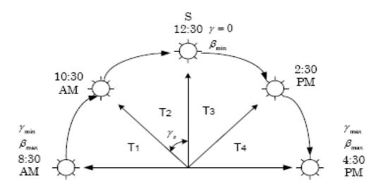
Figure 4. The division of daylight time into four intervals
