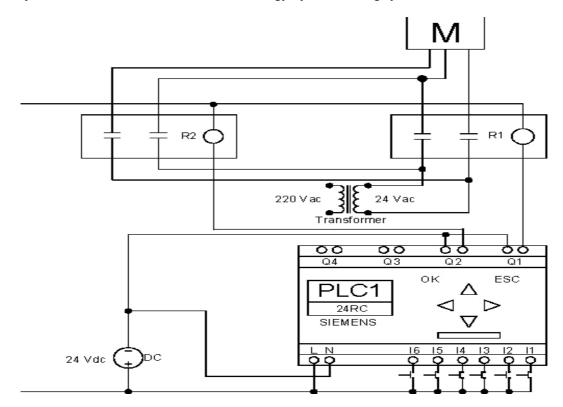
Figure 3. The electromechanical circuit for vertical control. 'Software used Microsoft Visio'
