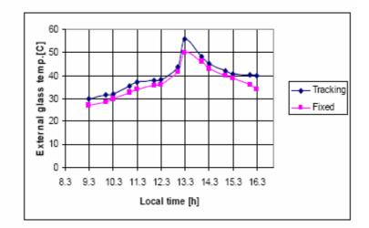
Figure 6. Temperature variation of pot water for both fixed cooker and sun tracked solar cookers
