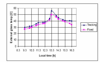
Figure 7. Temperature variation of the external glass for both fixed cooker and sun tracked solar cooker
