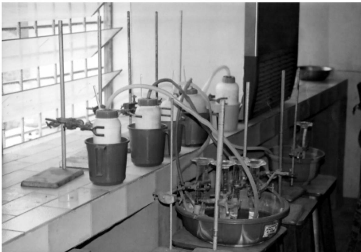
Figure 2. Experimental set-up for the laboratory scale biogas production
