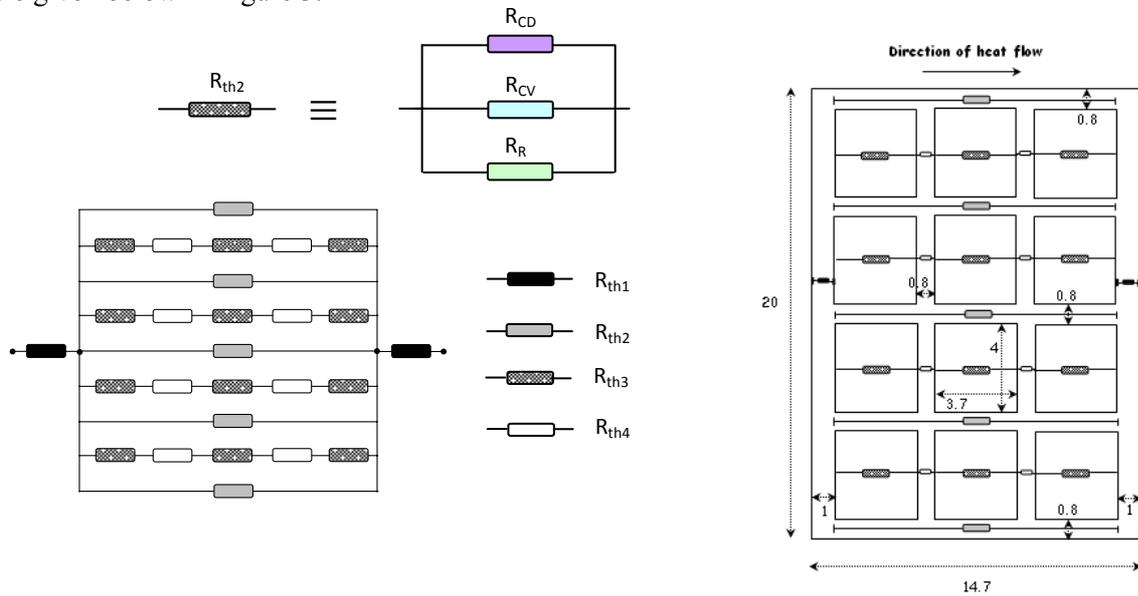
Figure 3. Dimensions (in centimeters) and equivalent circuit of a hollow brick
