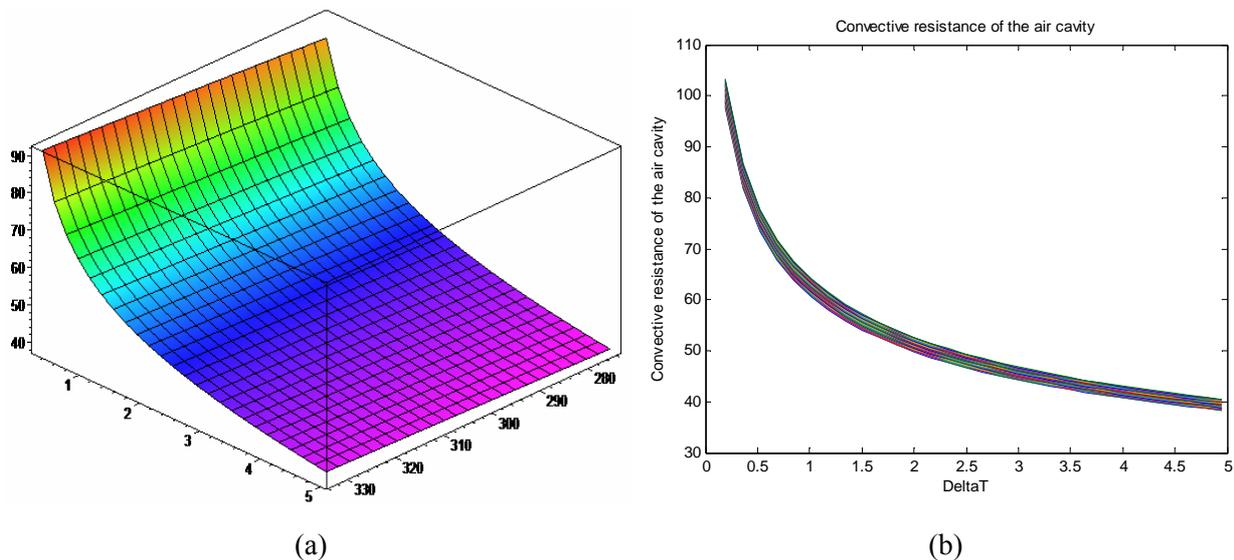
Figure 4. (a) variation of  $R_{CV}$  as function of  $T$  and  $\Delta\theta$ ; (b)  $R_{CV}$  as a function of  $\Delta\theta$  for  $T$  ranging from 0 to  $60^\circ\text{C}$
