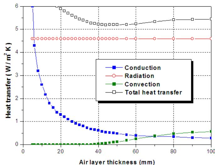
Figure 5. Estimated heat transfer in a closed air cavity bounded by ordinary materials  $\epsilon = 0.9$
