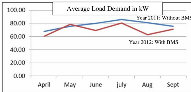
Figure 5. Effect of BMS in monthly average load demand in building No. 40
