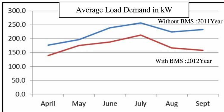
Figure 4. Effect of BMS on monthly average load demand in building No. 29
