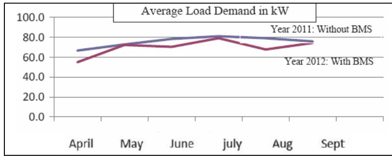
Figure 6. Effect of BMS in monthly average load demand in building No. 51
