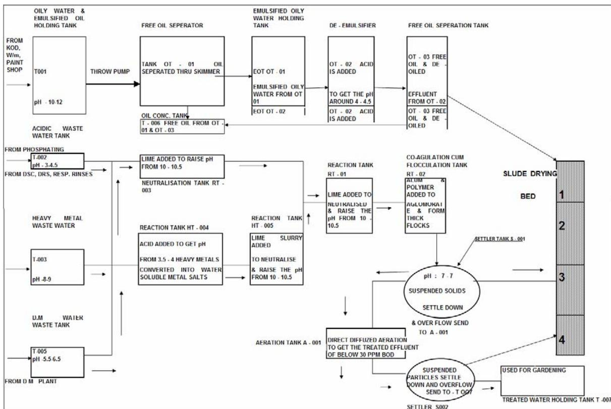
Figure 1. Flow diagram of effluent treatment plant
