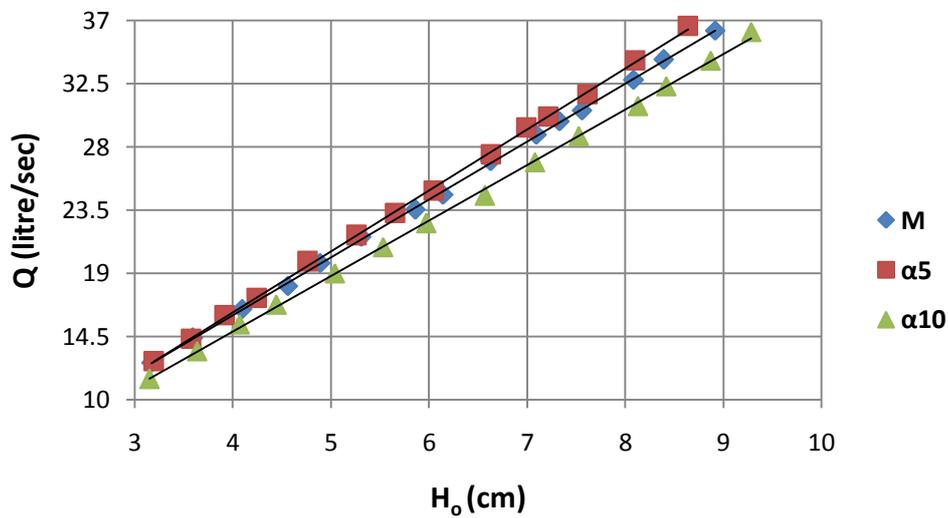
Figure 5. Experimental rating curves for models (M), ( $\alpha 5$ ), and ( $\alpha 10$ )
