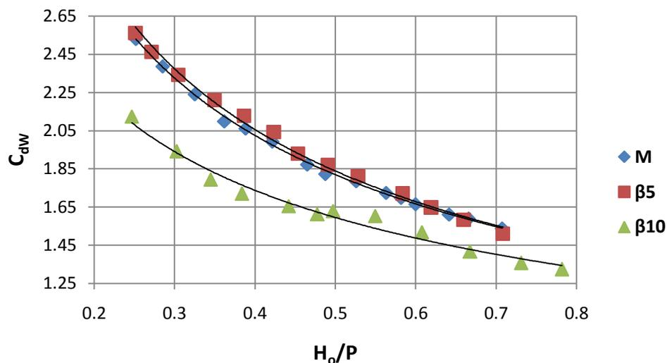
Figure 8. Variation of  $C_{dw}$  vs.  $H_o/P$  for three  $\beta$  values
