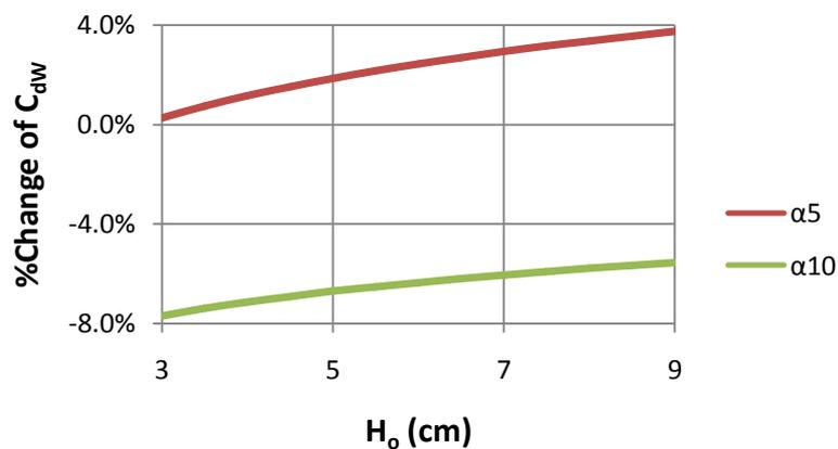
Figure 6. Percentage change of  $C_{dW}$  for the ( $\alpha 5$ ) and ( $\alpha 10$ ) relative to model (M) vs.  $H_o$
