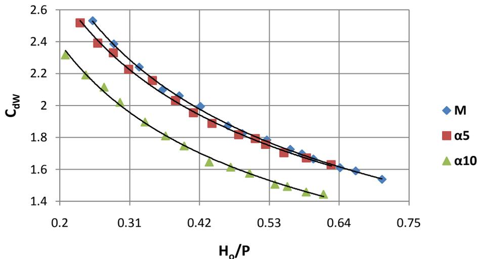
Figure 3. Variation of  $C_{dW}$  vs.  $H_o/P$  for three  $\alpha$  values
