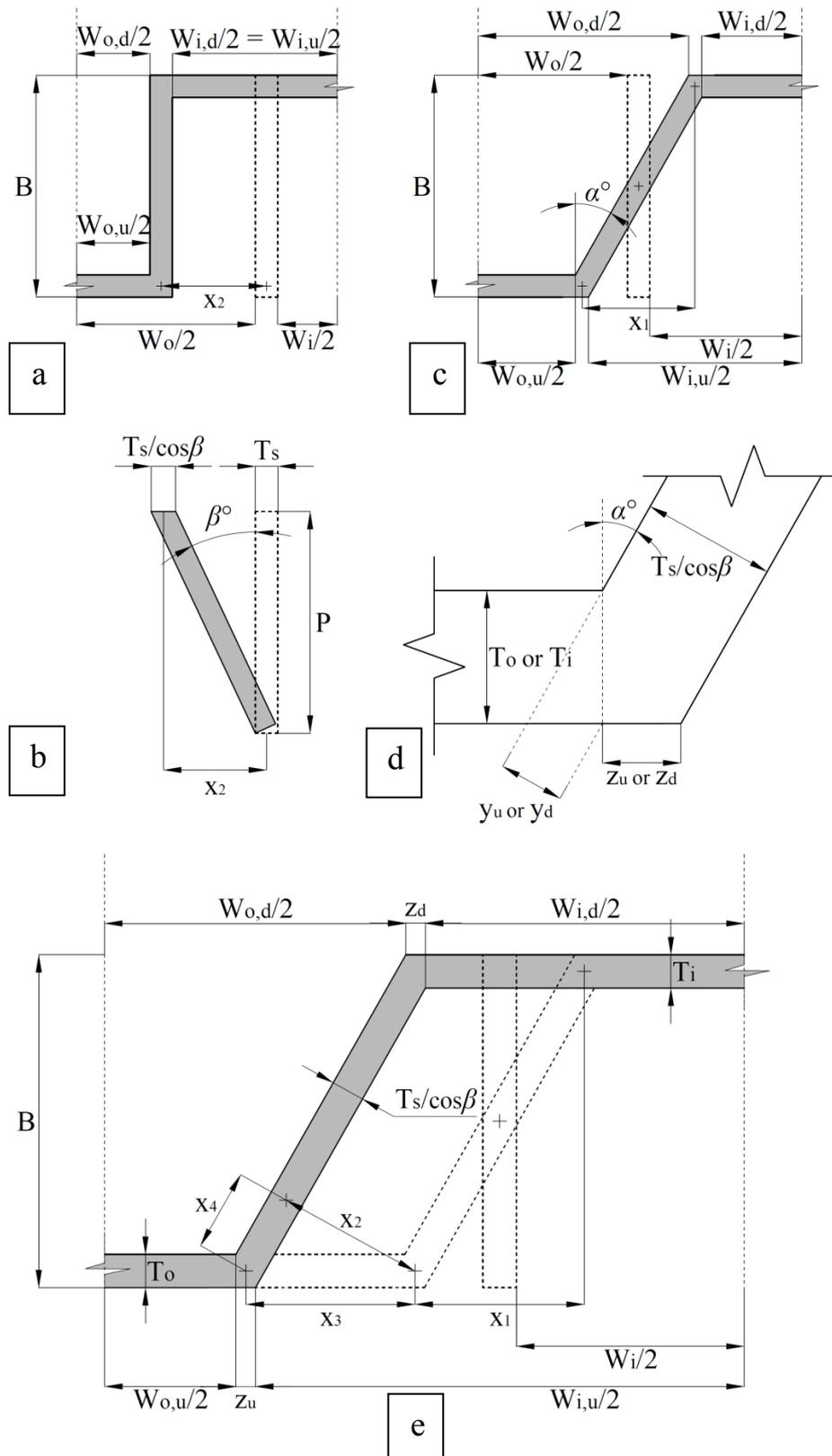
Figure 2. Half unit details of PKW with variations of angles  $\alpha$  and  $\beta$ . (a) Top-view,  $\beta > 0$  and  $\alpha = 0$ , (b) Front-view,  $\beta > 0$  and  $\alpha = 0$ , (c) Top-view,  $\alpha > 0$  and  $\beta = 0$ , (d) Details of crest thickness at the transition between inlet (or outlet) key crest and side crest, and (e) Top-view,  $\beta > 0$  and  $\alpha > 0$
