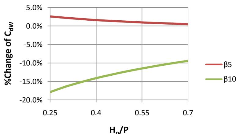
Figure 9. Percentage change of  $C_{dw}$  for the  $\beta$  models relative to model (M) vs.  $H_o/P$
