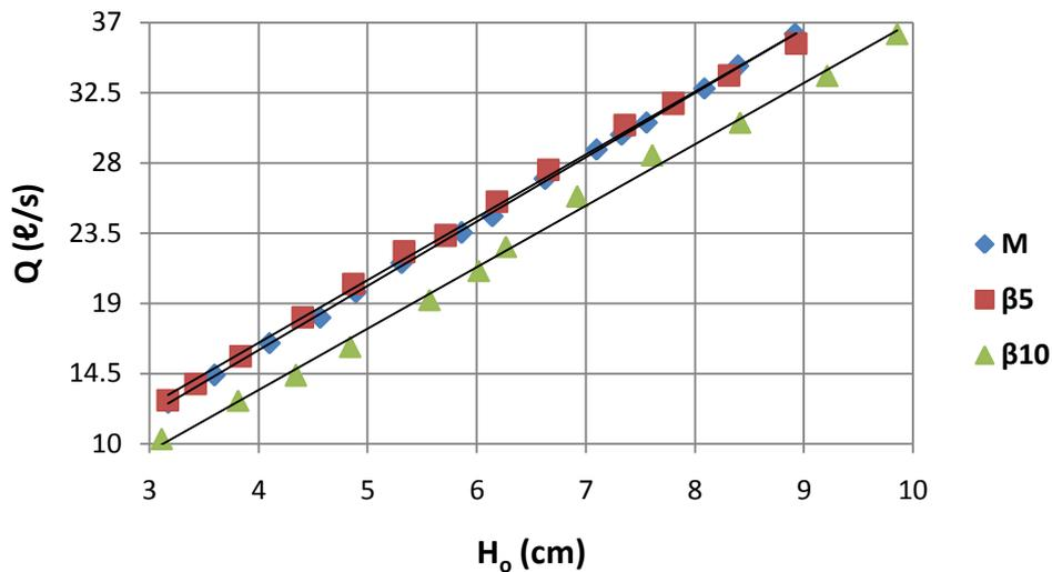
Figure 10. Experimental rating curves for models (M), ( $\beta 5$ ), and ( $\beta 10$ )
