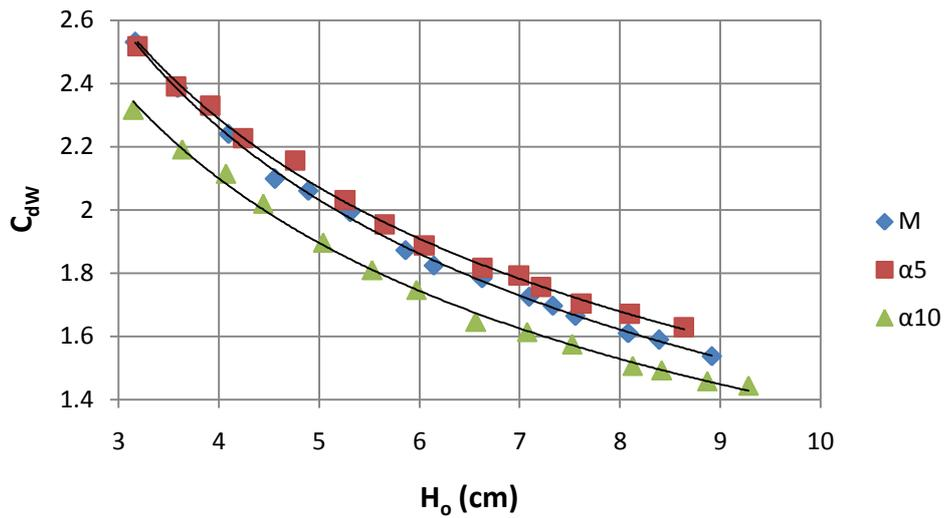
Figure 4. Variation of  $C_{dW}$  vs.  $H_o$  for three  $\alpha$  values
