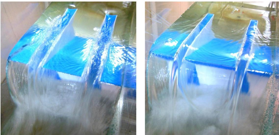
Figure 11. Views of PKW models ( $\beta 5$ ) (left), and ( $\beta 10$ ) (right)
