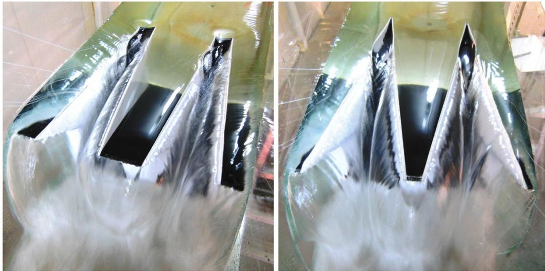
Figure 7. Views of PKW models ( $\alpha 5$ ) (left), and ( $\alpha 10$ ) (right)
