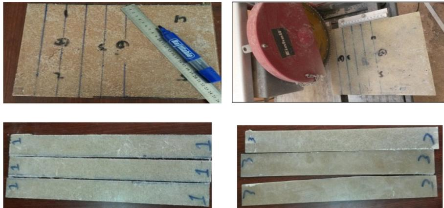
Figure 5. Tensile test samples preparing
