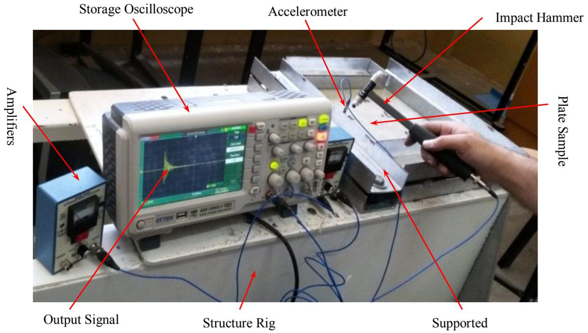
Figure 12. Rig and vibration test machine of composite plate structure
