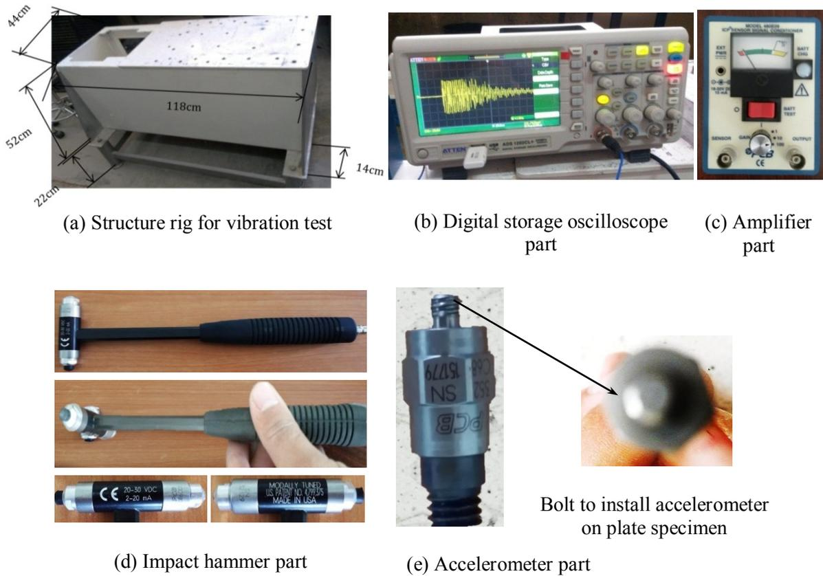
Figure 13. Vibration test machine parts
