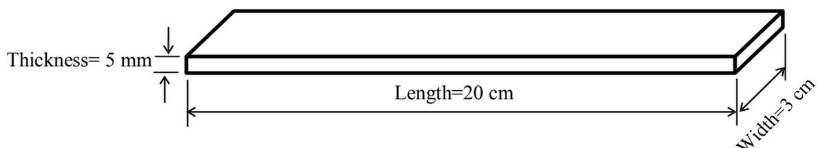
Figure 4. Shape and dimensions of tensile test sample
