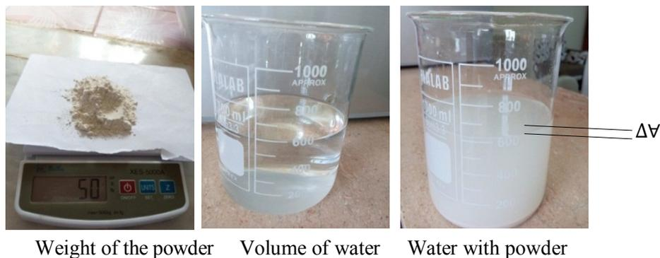
Figure 1. Steps to evaluate density of glass powder used
