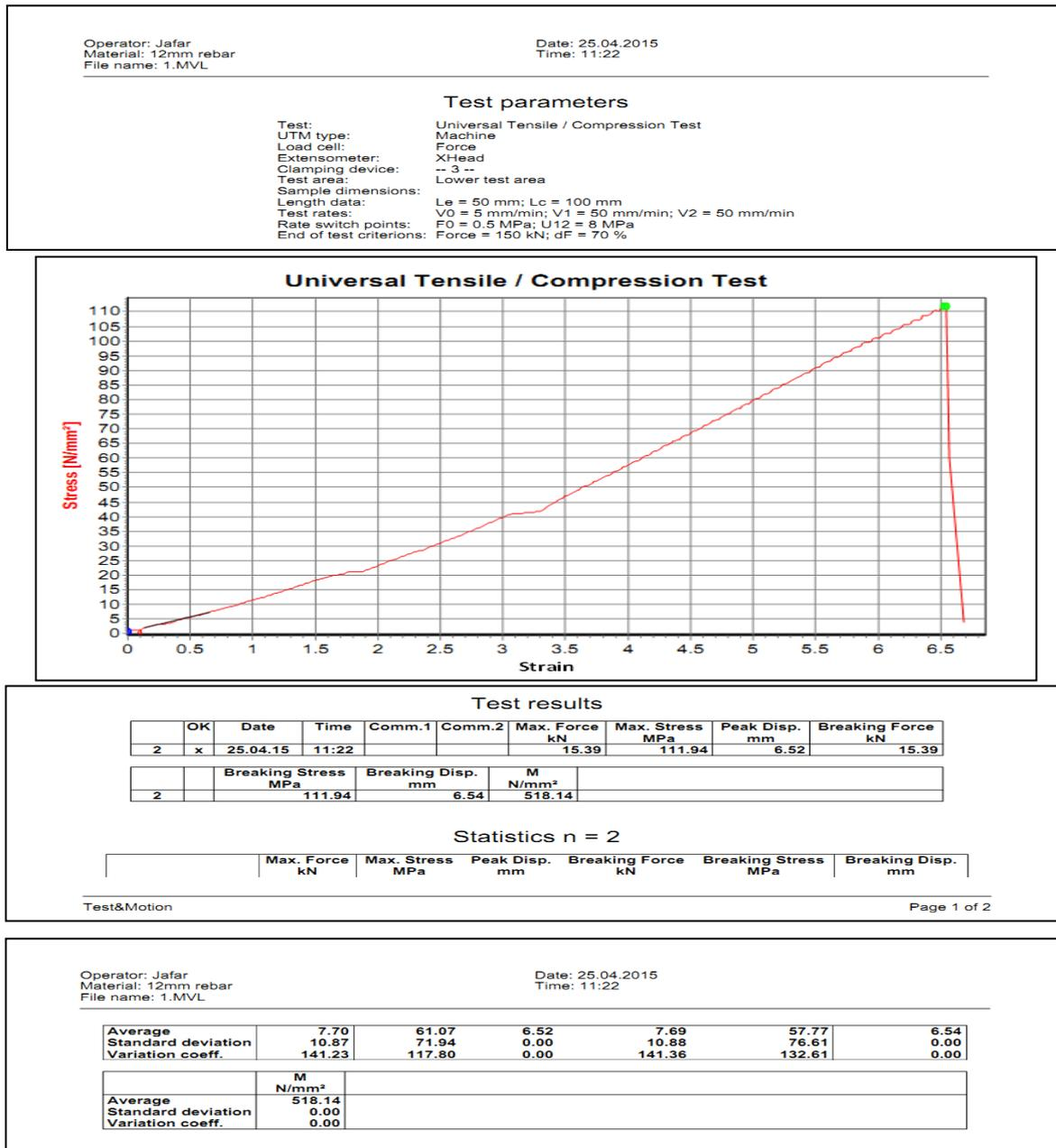
Figure 8. Tensile test result of short reinforcement glass fiber, glass reinforcement powder, and epoxy resin composite (sample 5)
