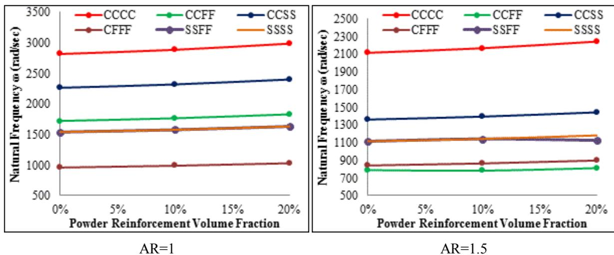
Figure 20. Experimental natural frequency with powder reinforcement effect and various plate boundary condition, for short fiber volume fraction  $V_{sf} = 30\%$  and various plate aspect ratio
