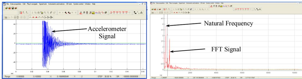
Figure 17. Sig-view program for FFT analysis function
