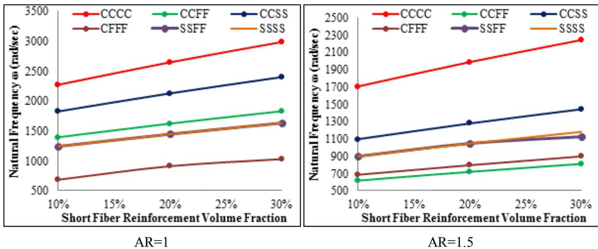
Figure 22. Experimental natural frequency with reinforcement short fiber effect and various plate boundary condition, for powder reinforcement volume fraction  $V_{pf} = 20\%$  and various aspect ratio
