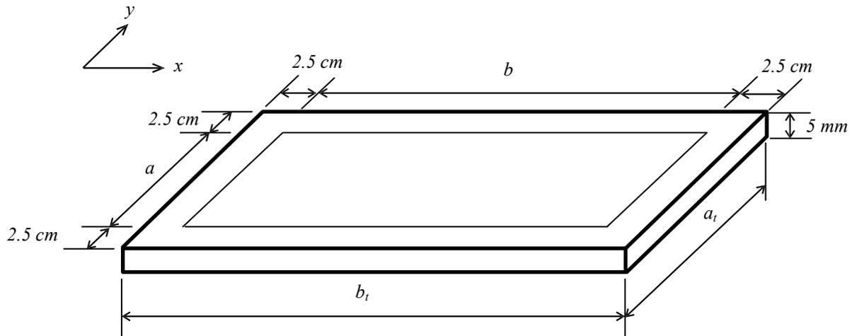
Figure 9. Shape and dimensions of vibration test sample
