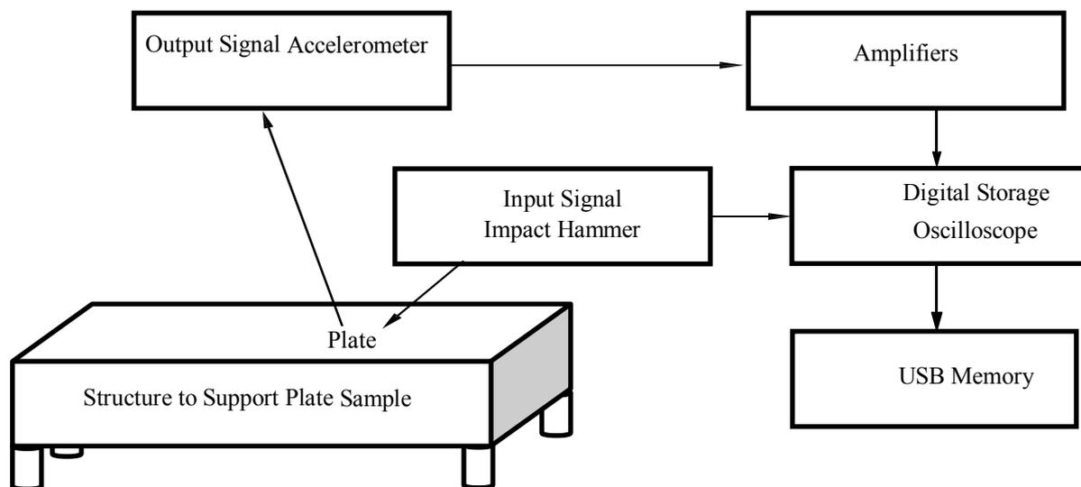
Figure 11. Flowchart of vibration structure rig
