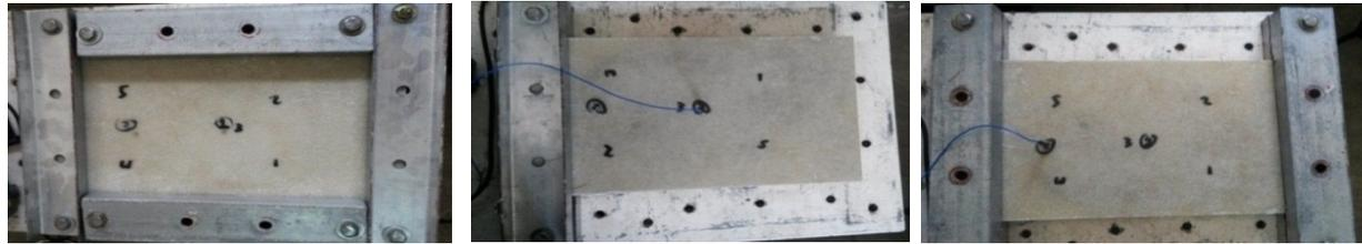
(b) Fixed the Accelerometer Part and impact location point for various boundary conditions of plate sample
