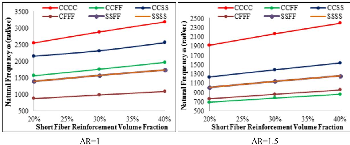
Figure 21. Experimental natural frequency with reinforcement short fiber effect and various plate boundary condition, for powder reinforcement volume fraction  $V_{pf} = 10\%$  and various aspect ratio
