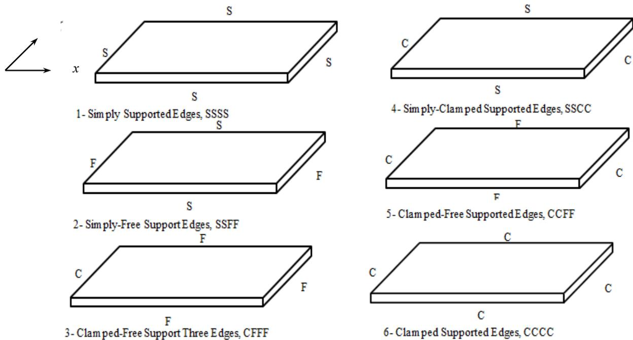
Figure 10. Different boundary conditions of vibration test plate
