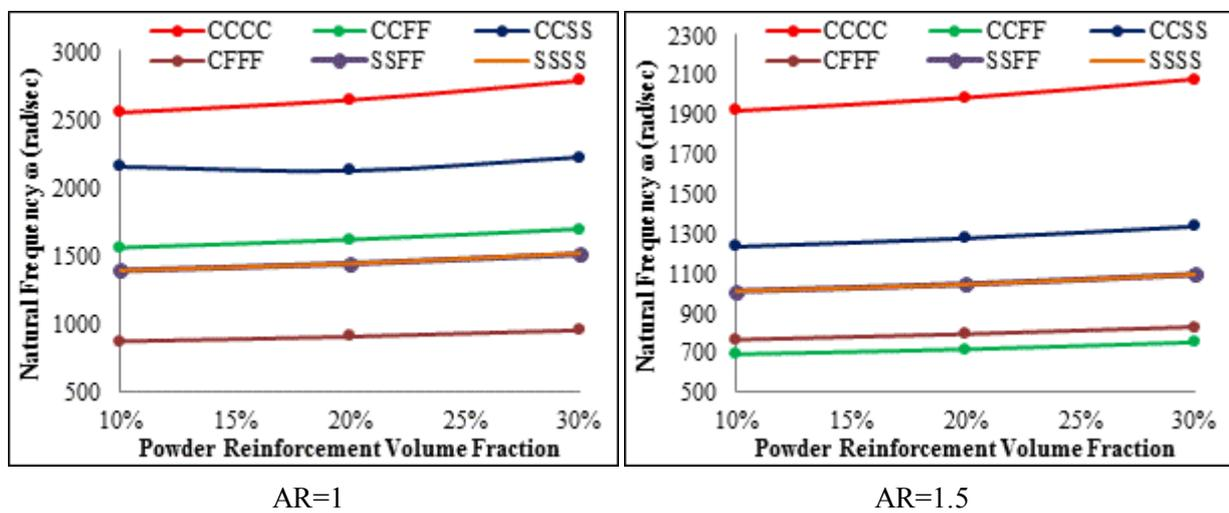
Figure 19. Experimental natural frequency with powder reinforcement effect and various plate boundary condition, for short fiber volume fraction  $V_{sf} = 20\%$  and various plate aspect ratio
