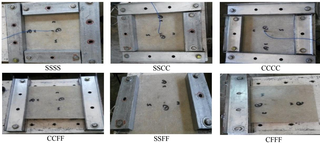
Figure 15. The vibration test composite plates with different boundary conditions
