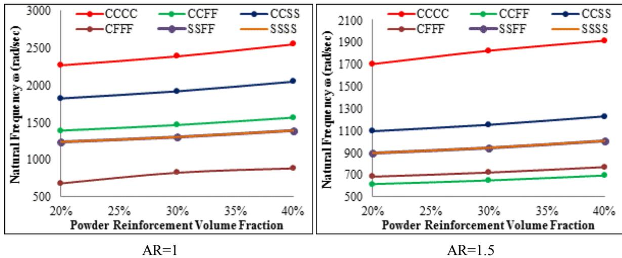
Figure 18. Experimental natural frequency with powder reinforcement effect and various plate boundary condition, for short fiber volume fraction  $V_{sf} = 10\%$  and various plate aspect ratio
