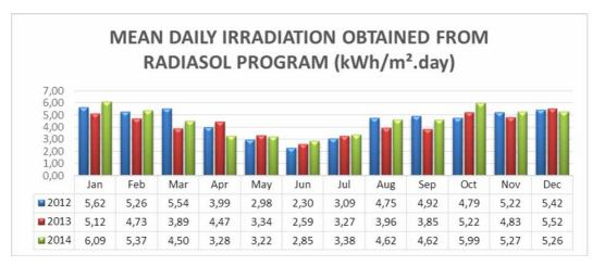
Figure 6. Mean daily irradiation on GO's PV panel surface obtained from RADIASOL software (kWh/m<sup>2</sup>.day). Source: The authors.
