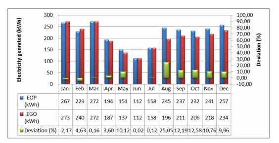
Figure 7. Comparison between the optimum grid-connected PV system and the real GO's grid-connected PV in 2012. Source: The authors.
