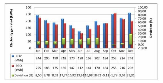
Figure 9. Comparison between the optimum grid-connected PV system and the real GO's grid-connected PV in 2013. Source: The authors.
