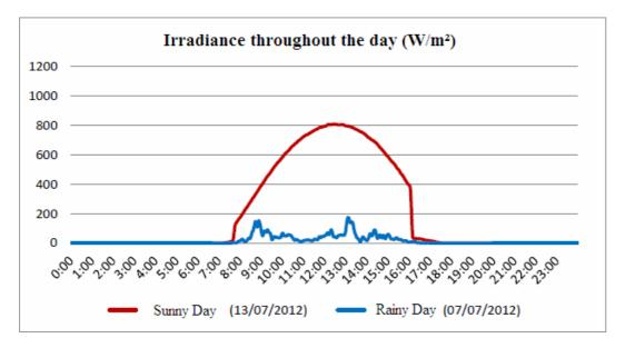
Figure 12. Irradiance curves obtained at panel surface in July [19].
