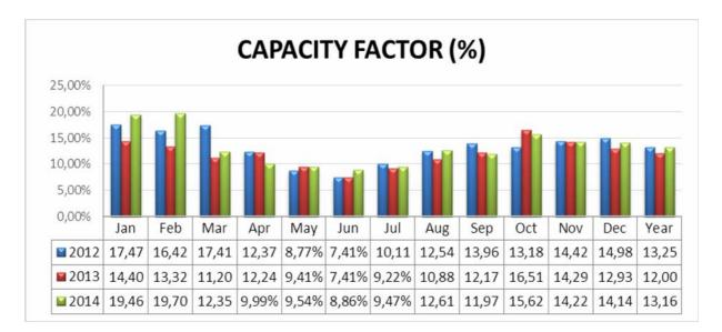
Figure 14. Monthly and annual Capacity Factor of the GO's grid-connect PV system of the UTFPR. Source: The authors.
