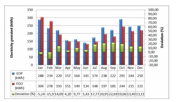
Figure 10. Comparison between the optimum grid-connected PV system and the real GO' grid-connected PV in 2014. Source: The authors.
