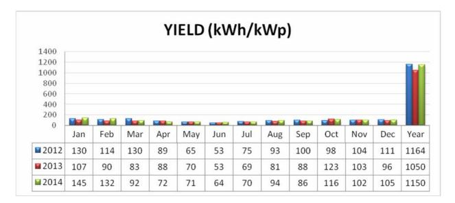
Figure 11. Monthly and annual Yield of the GO's grid-connect PV system of the UTFPR. Source: The authors.
